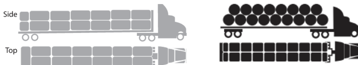
Figure B-5. Square and round Bale stack configuration on a 53-ft flatbed trailer truck
